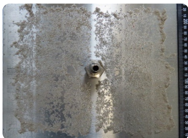
Figure 10. Coarse (above) and fine (below) rejects on the screening plates
