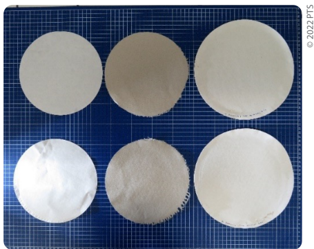
Figure 35. Hand sheets analysed in the sheet adhesion test with incident light
